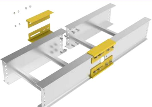
Optional quarter-span Support Reduction Expansion Couplers can be placed within the quarter span position without supporting both sides of the joint. These couplers can reduce the cost of installation by reducing the number of supports needed. Bonding jumpers are required.
