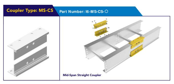
Optional mid-span couplers can be placed at any location within a span, eliminating the need to have couplers located within the quarter span position as shown in NEMA VE-2. This can reduce the number of supports required and cost of installation.
