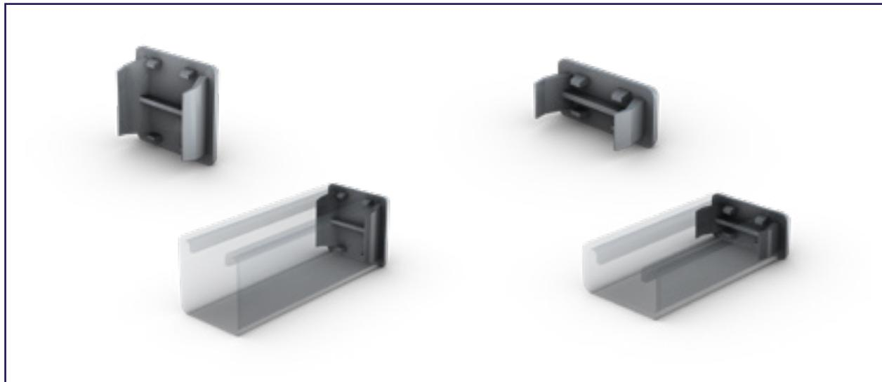
Protective End Caps are designed to close off the open ends of Intelok Deep and Shallow Channel Profiles. End caps are also used with Intelok Concrete Inserts to prevent the ingress of concrete slurry during the pouring process. Manufactured from injection moulded PVC, end caps are available in black or white colours.
