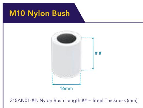
The length of the nylon bush is equal to the thickness of the supporting steelwork (##). The nylon bush requires a 17mm diameter hole in the supporting steelwork.
